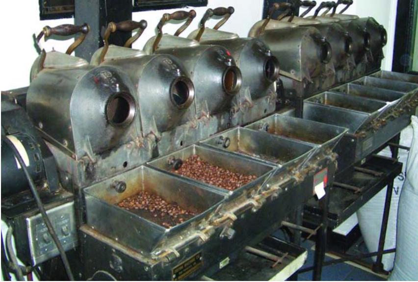
Tiny roasting machines are used to roast samples of different coffees to determine the particular flavor qualities of each one.
